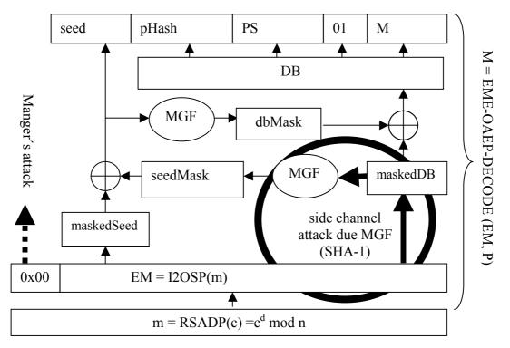
Fig.1: New side channel attack against RSA-OAEP
