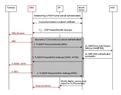
Figure 7: Man-in-the-Middle in PEAP, e.g., with EAP AKA
