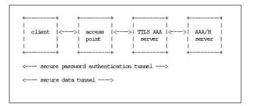
Figure 4: The network architectural model for EAP-TTLS [5]
