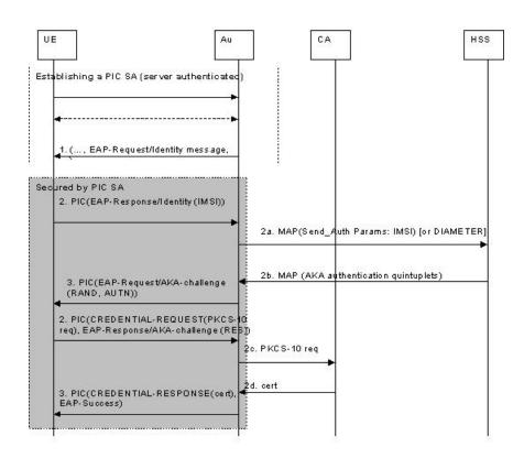
Figure 6: PIC with EAP AKA: Example Message Flow
