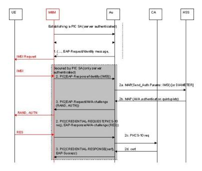
Figure 8: Man-in-the-Middle in PIC, e.g., with EAP AKA
