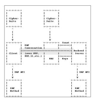
Figure 1: Relationship between EAP client, back-end authentication server and NAS in PEAP [1]
