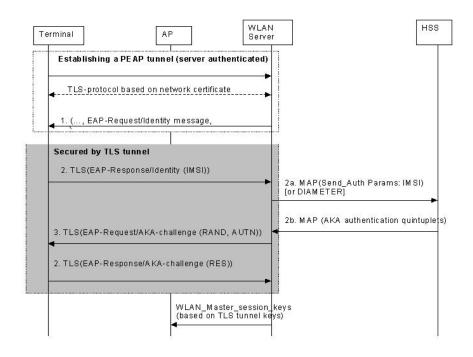
Figure 3: PEAP with EAP AKA: Example Message Flow
