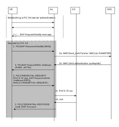
Figure 9: Binding for PIC and EAP AKA
