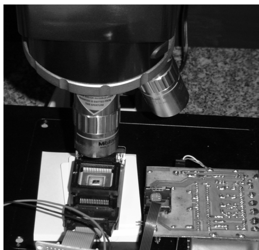
Figure 2. Laser Fault Injection Equipment (Inner View)
