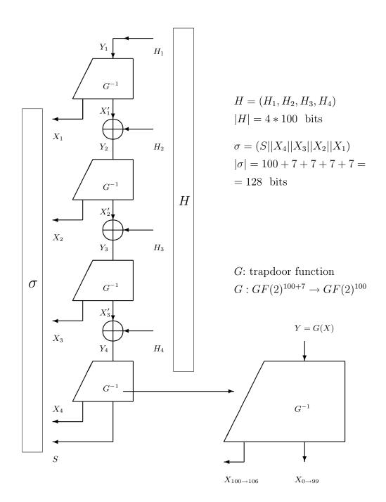
Fig. 4. Signature generation in Quartz
