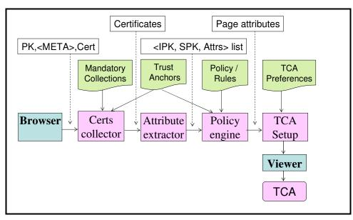
Figure 7: Determining the contents of the Trusted Credentials Area.
