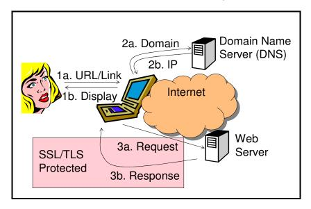
Figure 3: HTTP request/response process with SSL protection
