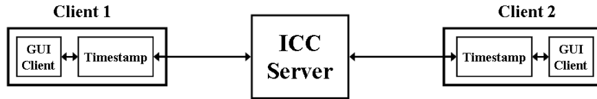
Figure 2: The ICC configuration: clients communicate through a timestamp process which records the arrival-time of incoming moves and computes the elapsed time for a player’s move before transmitting it to the server. The timestamp process can be run on a different machine, but it is most often on the local machine. Some clients have the timestamp process built-in; this is the case with the Blitzin Windows client but not with any of the Unix clients.
