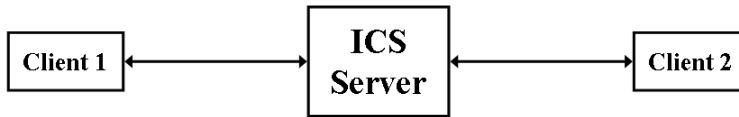
Figure 1: The original ICS configuration: clients made a TCP/IP connection to a port on a server. The ICS server enforced the rules of chess and maintained the state of each player’s clock. In this configuration, network lag would be charged to the players’ clocks.
