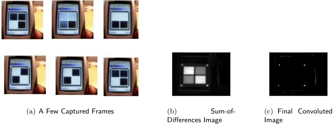
Figure 7: An example of various images in the decoding process (with 4 slots per frame)
