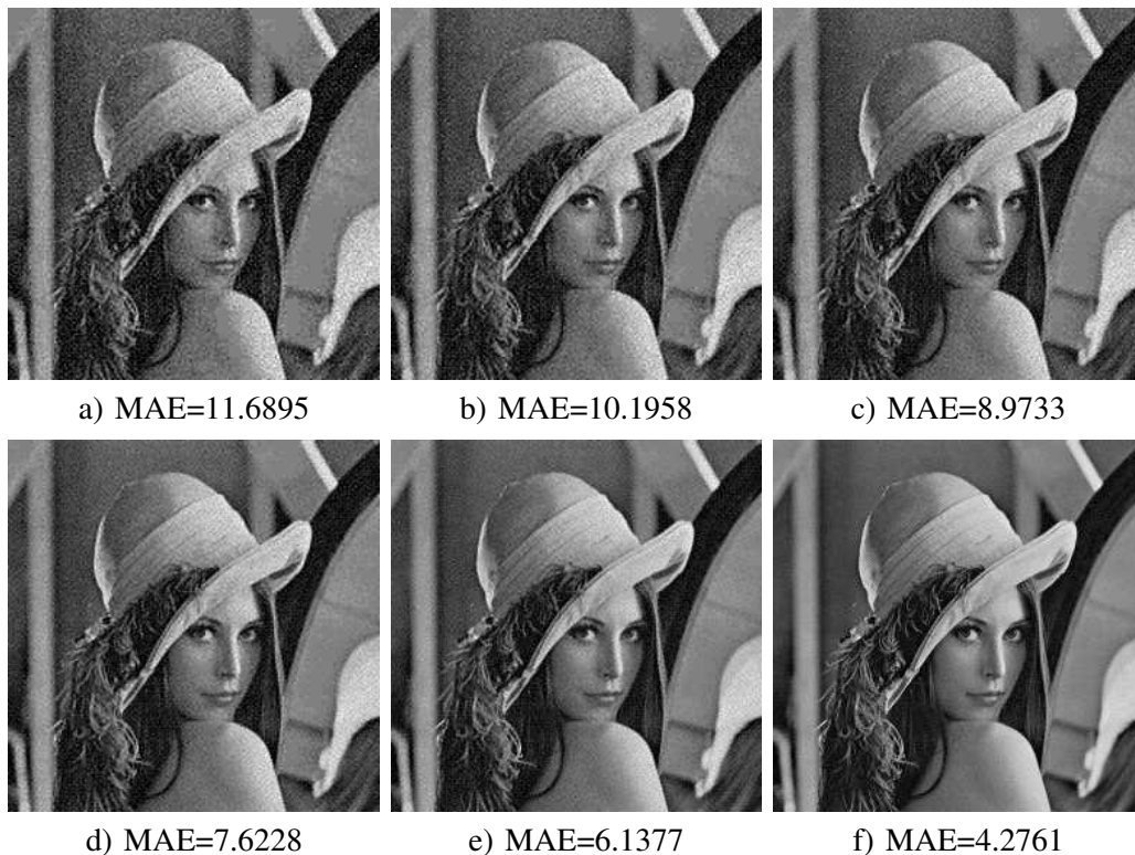
Fig. 22. The lossy decryption results when the cipher-image Fig. 2b is compressed by the standard JPEG algorithm: a) Quality=40; b) Quality=50; c) Quality=60; d) Quality=70; e) Quality=80; f) Quality=90.
