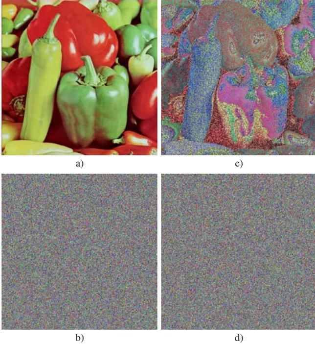
Fig. 1. Low sensitivity with respect to plain-image: a) plain-image “Peppers”, b) the encryption result of Fig. 1a), c) the masked version of Fig. 1a) with a random  $\{0, 128\}$  binary image, d) the encryption result of Fig. 1c).
