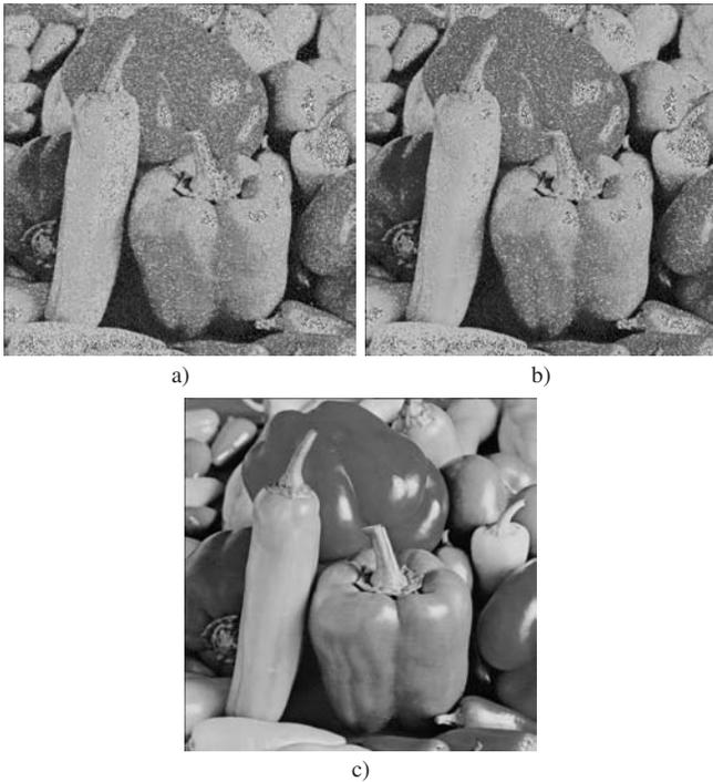
Fig. 7. The result of chosen plain-image attack (red channel): a) one chosen plain-image of fixed value 43; b) two chosen plain-images of fixed value 43, 53; c) three chosen plain-images of fixed value 43, 53, 85.
