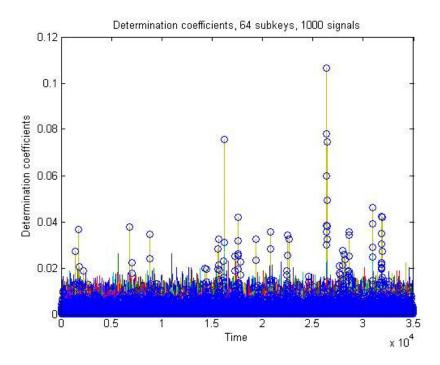
The attack is clearly successful: we have significant correlation/determination peaks for one and only one particular value of the subkey (in yellow) which is the true value  $k_0$  (blue circles). With the same data, the Bayes Factors procedure gives, in logarithmic scale
