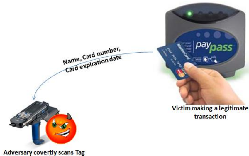
Fig. 4. An eavesdropping attack on an RFID enabled Credit Card
