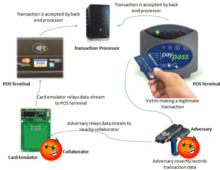
Fig. 5. A relay attack on an RFID enabled Credit Card
