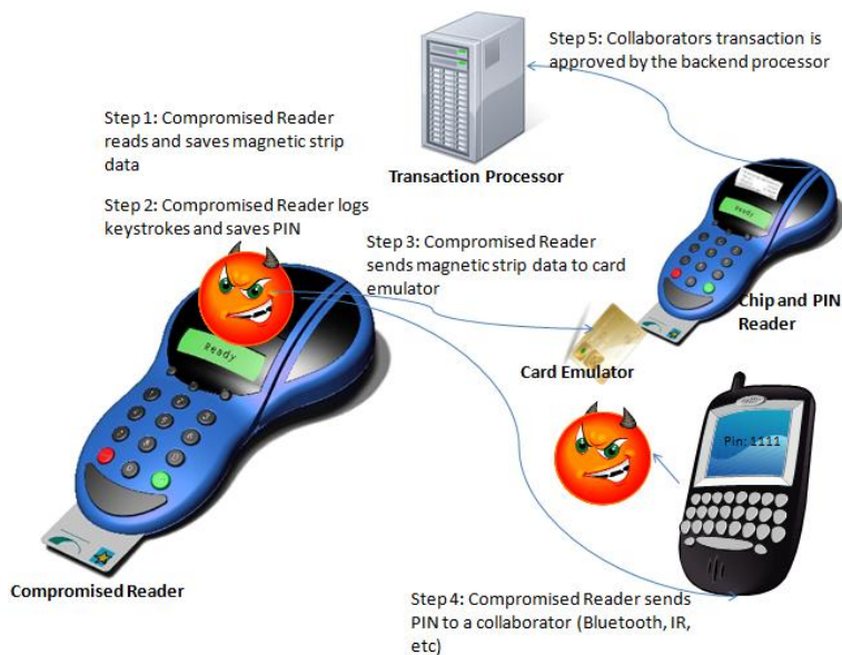
Fig. 2. A PIN and Chip based relay attack
