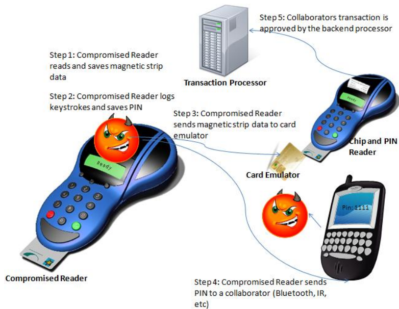
Fig. 1. A PIN and Chip based relay attack
