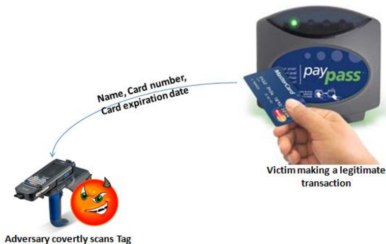
Fig. 2. An eavesdropping attack on an RFID enabled Credit Card
