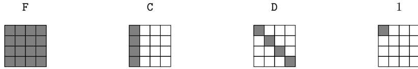
Fig. 2. Notations for byte-wise truncated differential states for one word of ECHO. Each cell represents a byte and a gray cell stands for an active byte.
