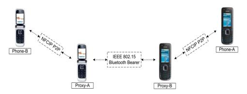
Fig. 1. P2P Relay Setup using Bluetooth.
