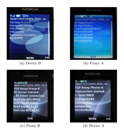
Fig. 3. Relay attack data flow on each device involved.
