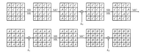
Fig. 2. The development of a  $\delta$ -set through 3 rounds of AES, where A stands for an active byte, B stands for a balanced byte, and C stands for a constant byte
