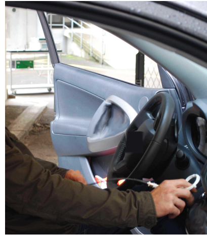
(b) Starting the engine using the relay
