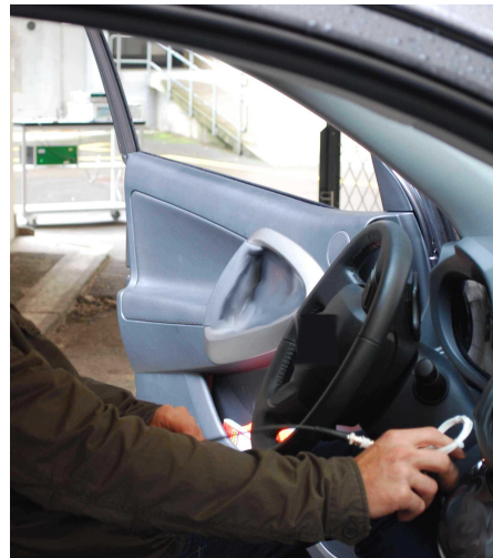
(b) Starting the engine using the relay.
