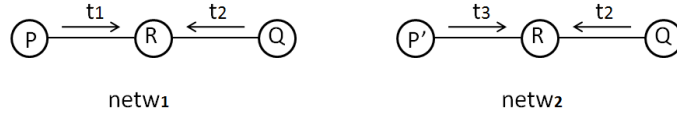
Figure 8: The two networks netw_1 and netw_2 have the same topology but the operations of the leftmost nodes differ (P and P').
