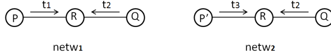
Figure 8: The two networks netw_1 and netw_2 have the same topology but the operations of the leftmost nodes differ (P and P').
