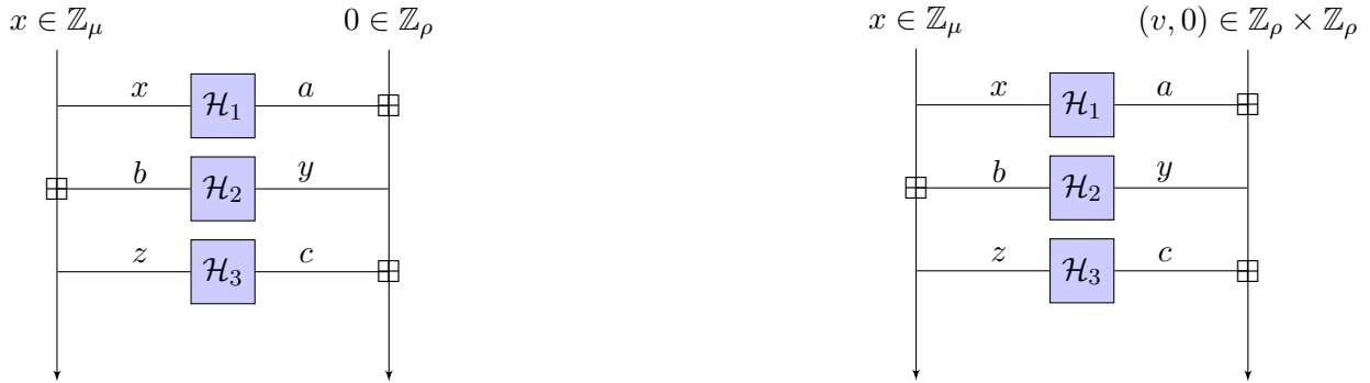
Figure 2: (left) An unbalanced three-round Feistel network \phi_{3f} over \mathbb{Z}_\mu \times \mathbb{Z}_\rho . (right) The three-round Feistel network \phi_{3F} with an extra \mathbb{Z}_\rho domain on the right side. These permutations define evaluation functions of padding schemes \pi_{3f}(x) = \phi_{3f}(x, 0) and \pi_{3F}(x, v) = \phi_{3F}(x, v, 0) by fixing the rightmost \mathbb{Z}_\rho part of the input to 0.
