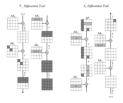
Fig. 2. Differential trails for a four round biclique of mCrypton-96 according to key differences  $\nabla_i^K$  (left) and  $\Delta_i^K$  (right).
