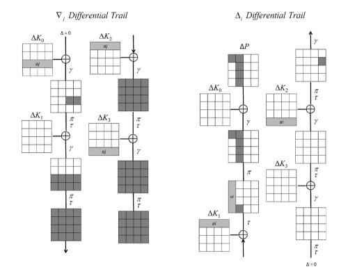
Fig. 5. Differential trails for a four round biclique of mCrypton-128 according to key differences  $\nabla_i^K$  (left) and  $\Delta_i^K$  (right).
