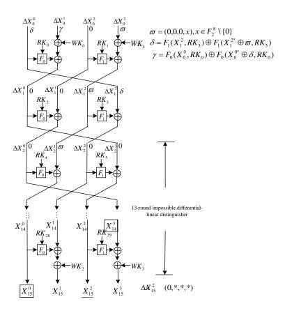
Fig. 7. 15-round impossible differential-linear attack
