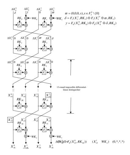
Fig. 3. 16-round impossible differential-linear attack
