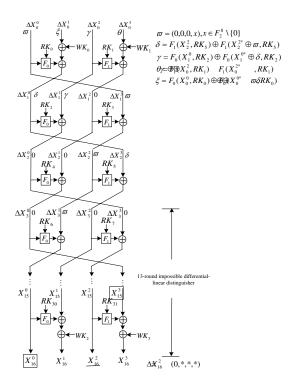
Fig. 5. 16-round impossible differential-linear attack
