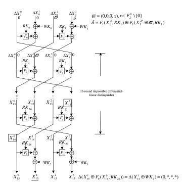
Fig. 6. 15-round impossible differential-linear attack
