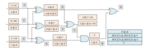
**Fig. 5.** An attack on GaX with DKC  $\mathbb{E}(A, B, T, X) = H(A[1: k-1] \parallel T) \oplus H(B[1: k-1] \parallel T) \oplus X$ . In each wire, the top token has semantics 0, the bottom one has semantics 1. The table on the right is the garbled table of gate 8. Gate 9 negates the bit on wire 4, then ORs it with the bit on wire 8.
