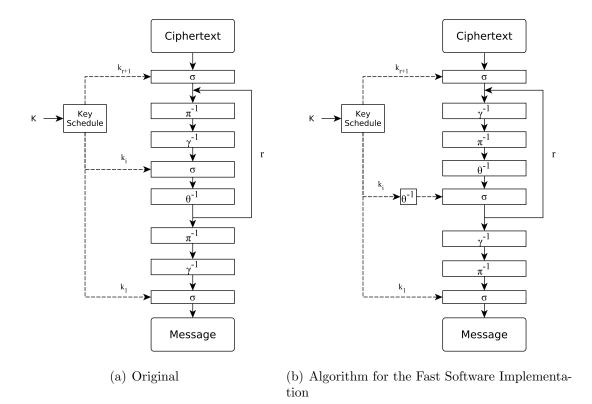
Figure 3: Decryption Algorithm of AES
