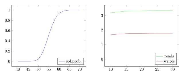
The left plot above shows the probability of finding a 42-cycle as a function of the percentage edges/nodes, as determined from 10000 runs at size  $2^{20}$ . The right plot shows the average number of memory reads and writes per edge as function of log size, as determined from 1000 runs each. It is almost constant at 3.3 reads and 1.75 writes.
