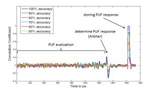
Fig. 4. The correlation of responses with different accuracies with 2000 simulated power traces of a 128-bit Arbiter PUF.
