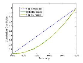
Fig. 8. Relation between the correlation coefficient and the prediction accuracy for the Hamming weight power model as well as the Hamming distance power model. For this simulation 1 million random response bits were used and no noise was added.
