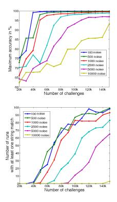
Fig. 9. Result of of 100 runs of an 80-bit CCMA-ES attack with different levels of noise. The noise level is expressed by the number of randomly switching registers that would generate the same amount of noise. On the left the maximum achieved accuracy with 100 runs is shown while on the right the number of runs that achieved an accuracy high enough to find at least one string match is shown.
