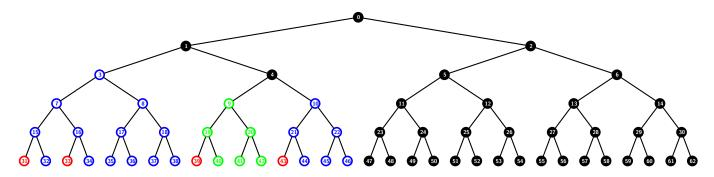
Figure 4: Example of a subset cover for  $\mathcal{R} = \{31, 33, 39, 43\}$  in the *a*-ABTSD scheme with a = 2 and n = 32 users. The subsets in the cover are  $S_{3,\{31,33\}}, S_{9,\{39\}}, S_{10,\{43\}}$  and  $S_{0,\{1\}}$ .
