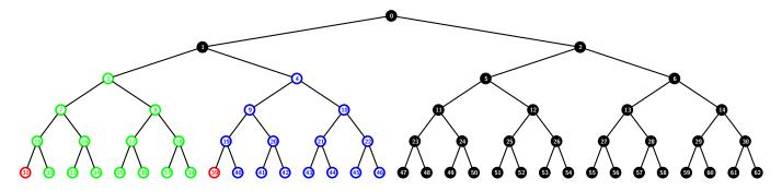
Figure 5: Example to show that the upper bound 2r-1 of the header length in the *a*-ABTSD scheme with a = 2 is tight. The subset cover for  $\mathcal{R} = \{31, 39\}$  in the binary tree  $\mathcal{T}^0$  with n = 32 users contains the subsets  $S_{3,\{31\}}$ ,  $S_{4,\{39\}}$  and  $S_{0,\{1\}}$ .
