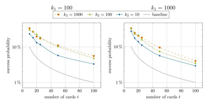
Figure 5: Simulations of the clustering attack for  $k_1$  (the number of samples during the fingerprinting phase) equal to 100 on the left and 1000 on the right, and varying values of  $k_2$  for each. The success probability, shown in log-scale, is averaged over fifty runs, and the simulation was done with t = 10, 15, 20, 25, 50, 100 cards. The baseline indicates the success probability of an adversary that tries to win the game by pure guessing.
