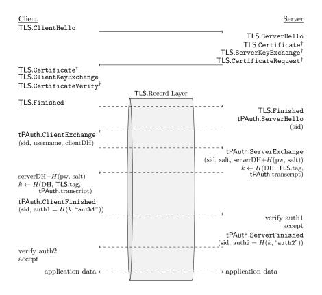
Figure 2: Protocol message diagram for TLS with tunnelled tag-based password authentication, with example messages for the tSOKE protocol. TLS.tag is either TLS.Finished or TLS.Certificate. <sup>†</sup> denotes optional messages.
