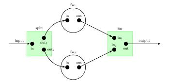
**Fig. 5.** The parallel composition of two firewalls with trusted hardware. hw only accepts packets that are output by both firewalls.
