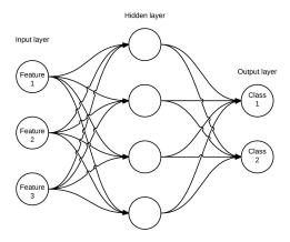
Figure 4. Representation of a simple neural network
