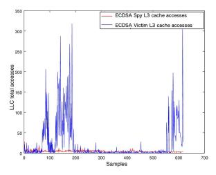
Figure 5. Total L3 cache accesses of spy and victim of the attack to ECDSA. The similarities are visible between samples 200 and 550 when the Montgomery ladder loop is executed.
