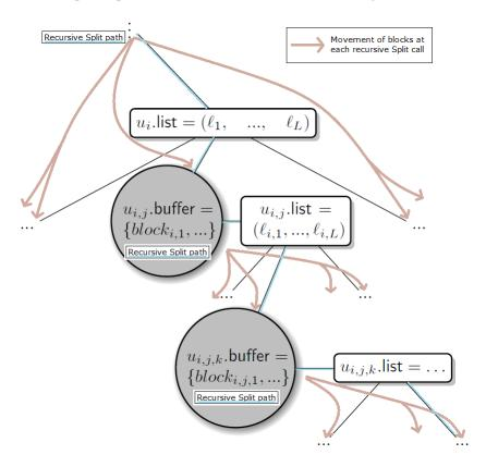
Figure 4: Internal blocks in subsequent splits of the server's tree T — i.e. "Flushing" (recursively).
