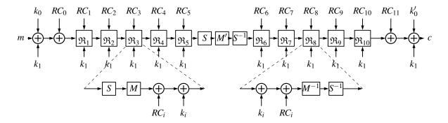
Fig. 1: The whole encryption process of PRINCE
