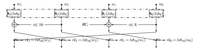
Fig. 8: One round key schedule of RECTANGLE-128, where  $lsb_n$  means taking the *n* least significant bits
