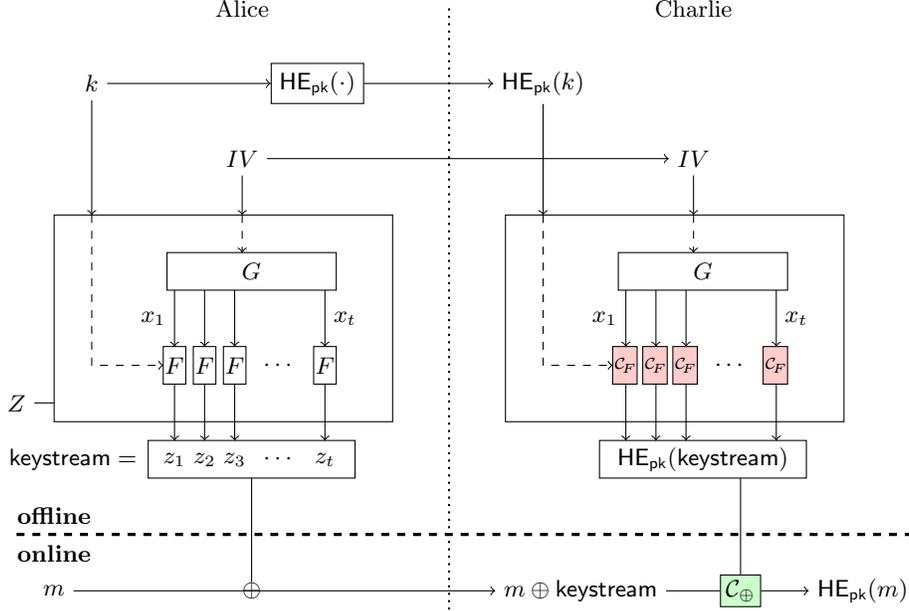
**Fig. 1.** Our generic construction. The multiplicative depth of the circuit is equal to the depth of  $\mathcal{C}_F$ . This will be the bottleneck in our protocol and we want the multiplicative depth of  $F$  to be as small as possible. With current HE schemes, the circuit  $\mathcal{C}_\oplus$  is usually very fast (addition of ciphertexts) and has a negligible impact on the noise in the ciphertext.
