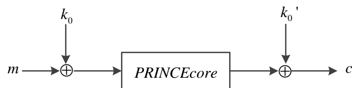
Fig1. The construction of PRINCE
