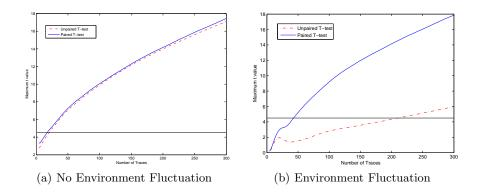
**Fig. 4.** T-test comparison for 1O leakage on unprotected Simon for a single measurement campaign of up to 300 pairs of traces. The paired t-test performs as well or better in both scenarios. However, the paired t-test is more robust to environmental noise.
