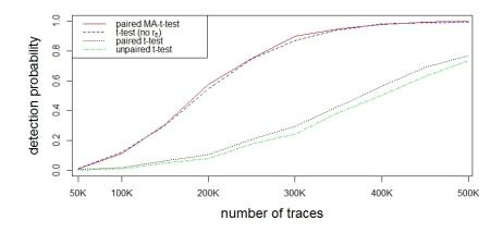
Fig. 3. T-test comparison for 2O leakage with a sinusoidal drift  $r_E$ .
