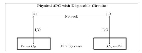
**Fig. 5.** Schematic of the physical setup for secure physical 2PC using disposable circuits (Protocol 2).
