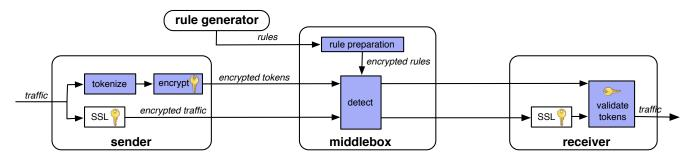
Figure 1: System architecture. Shaded boxes indicate algorithms added by BlindBox.
