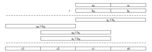
Fig. 1: The MOV-and-ADD coefficient multiplication.
