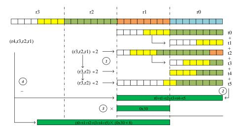
Fig. 4: Fast reduction operation with SMAS2 method for q=12289. ①: shifting; ②: addition; ③: multiplication; ④: subtraction.
