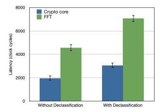
Figure 5: Latency measurement with the Trusted Wrapper
