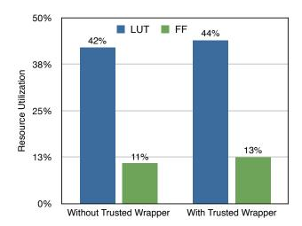
Figure 4: Resource utilization for an IP core with and without a Trusted Wrapper
