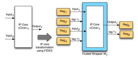
Figure 3: Trusted Wrapper mechanism for an IP Core
