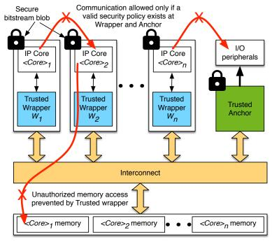
Physical memory partition based on IP core access labels
