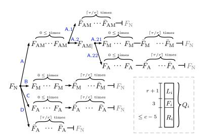
Fig. 4: The tree of all possible frame bits sequences for a single AD-message pair (top-left). The composition of an FDS query  $Q_i$  (bottom-right).
