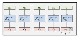
**Figure 3.2:** The OCB scheme illustrated for a four-block message  $M_1, \ldots, M_4$ , where  $\Sigma$  is the checksum  $M_1 \oplus \cdots \oplus M_4$ .
