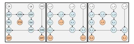
Figure 3.8: Left: An Enc graph that can be accepted or (incorrectly) rejected by Map, depending on the topological ordering of the nodes. Middle: The (type, ctr) pairs in each node of the Enc graph if the left TBC node is visited first. The graph is (incorrectly) rejected because the two OUT nodes both have ctr = 2. Right: The (type, ctr) pairs in each node of the Enc graph if the right TBC is visited first. This time, the graph is accepted because the two OUT nodes have different ctr values.
