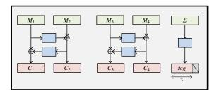
Figure 3.9: The OTR scheme, illustrated for a four-block message  $M_1 \cdots M_4$ . Here,  $\Sigma$  is the checksum of the even blocks  $M_2 \oplus M_4$ .
