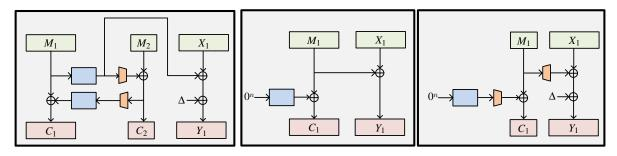
**Figure B.2:** Illustration of algorithm  $\sharp Enc$  when |M| > n (left), |M| = n (middle), or 0 < |M| < n (right). The incoming state  $X = X_1X_2$  and outgoing state  $Y = Y_1Y_2$ , with  $|X_i| = |Y_i| = n$ , will satisfy  $Y_2 = X_2$ , so we show only how to process  $X_1$  to get  $Y_1$ . The trapezoids represent truncation and padding with  $10^*$ .
