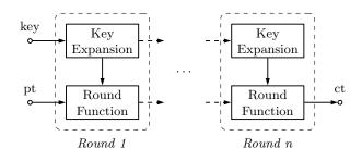
Fig. 1. Structure of unrolled block ciphers (pt: plaintext, ct: ciphertext).
