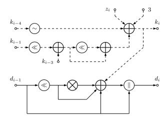
**Fig. 7.** Critical path diagram of one unrolled SIMON round ( $\sim$ : inverter,  $\ll$ : circular shift,  $z_i$ : bit from a predefined constant vector). The dashed part is the key expansion, which does not impact the critical path.
