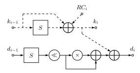
**Fig. 2.** Diagram of the critical of one unrolled AES round  $(RC_i: \text{round constant}, \ll: \text{circular shift}, \times: \text{finite field multiplier})$ . The dashed part is the key expansion, which does not impact the critical path.
