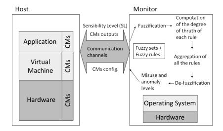
Fig. 14. Architecture of the prototype (hardware in dark grey, software in grey)
