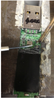
Fig. 4: Epoxy removal of Kingston DT 5000 with screwdriver
