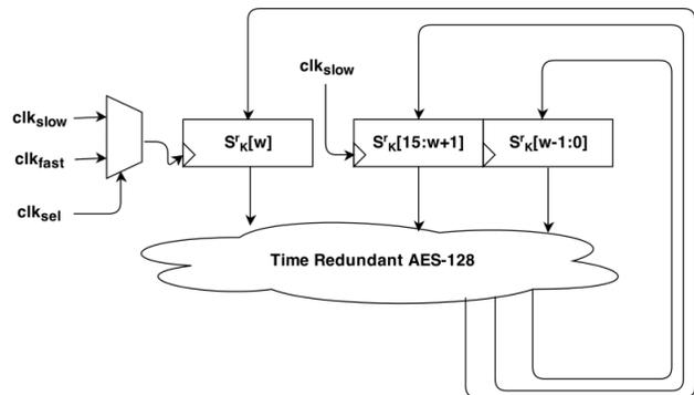
Fig. 9: Modified Fault Injection Setup: adversary has control over affected byte
