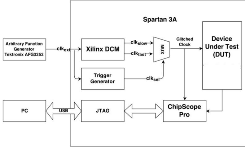
Fig. 2: Fault Injection Setup
