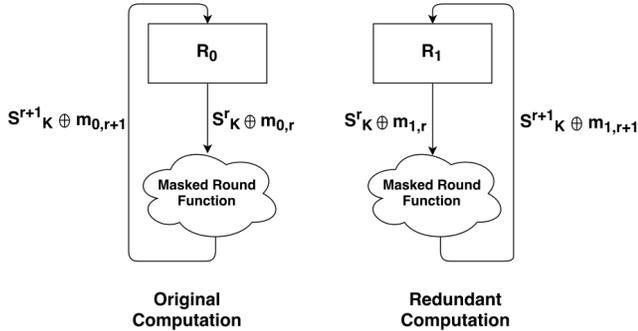
Fig. 5: A Schematic for the Masked Countermeasure
