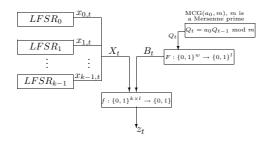
Figure 3: Proposed model for keystream generator
