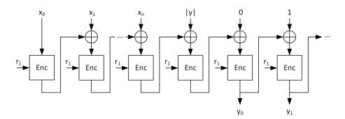
**Fig. 3.** PRF based on a block cipher in CBC mode. The variable-length message  $x_0, ..., x_n$  is expanded using a secret  $r_1$  into a message of length |y|
