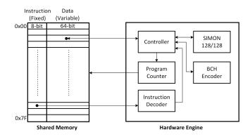
Fig. 7. Block Diagram of the Hardware Engine
