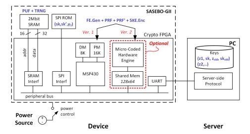
Fig. 6. System Architecture of the Device and Server
