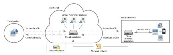
Figure 1: Network Function Virtualization.
